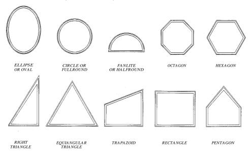
Shapes can be considered with respect to MULTILITE or MULTIPANEL formats (see Multiple Lite & Panel Format Section), shapes within shapes (ie. a standard rectangular shaped door with arched top panels) or over all unit shape (ie. Woodstone Fanlites).
